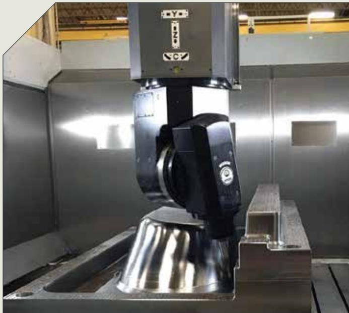
This image shows how the Parpas Diamond 30 features a generous table size for machining very large cavities and cores. With its orthogonally designed Model TOE-29 head that features a longer snout, it can reach into difficult-to-machine areas using shorter cutting tools. For Model Die and Mold, these capabilities have been a game changer by helping win new work and enabling more work done in-house.
